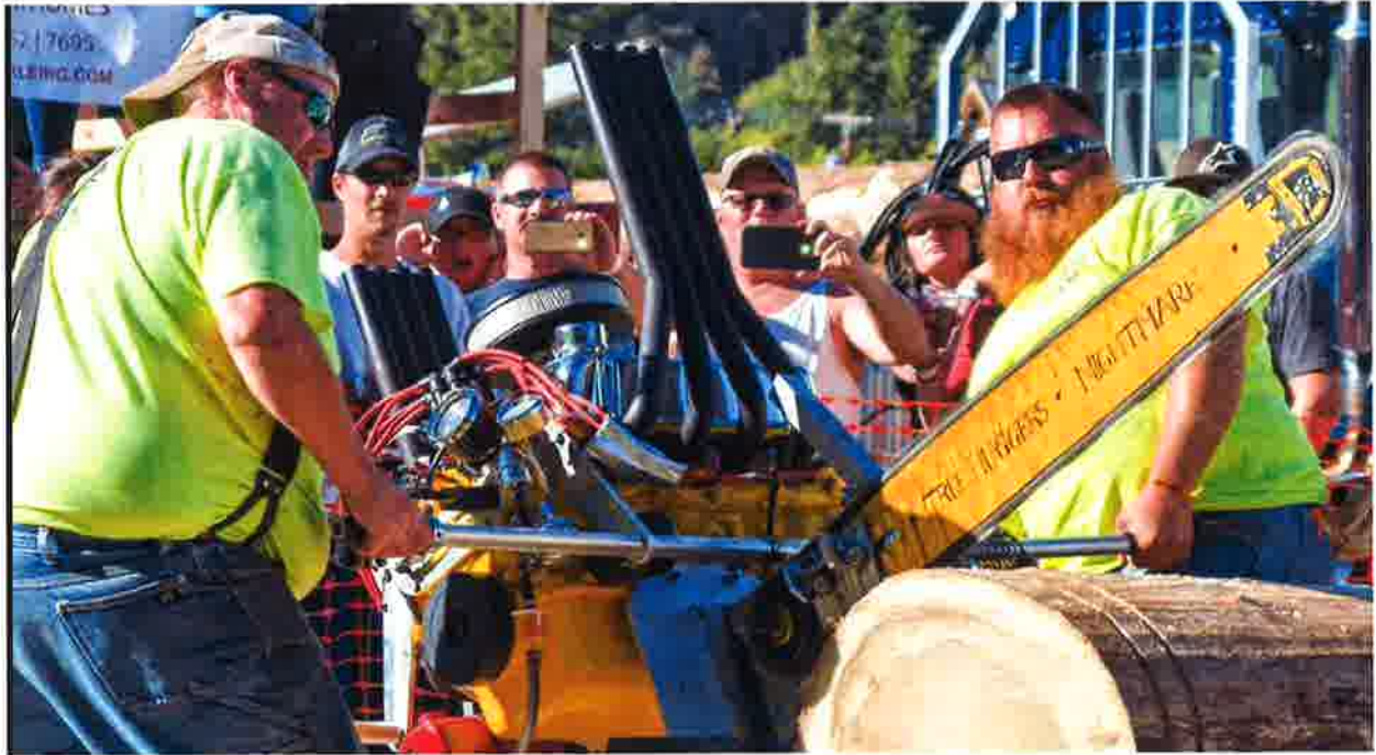
V8 Hotsaw (302 Ford) Car Engine Weighing 650 pounds
